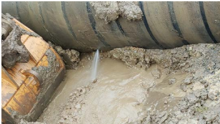
68 year old 45-inch Steel Pipe – localized corrosion failure
